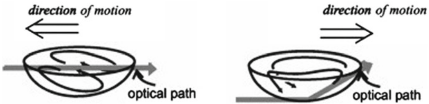
Fig. 13.3 Ways of illumination of a drop with alternative consequences (schematic). Light beam crossing a transparent drop midway (left panel) or by the side (lower panel). In the former the drop is pulled towards the light source while in the latter it is the opposite. Reprinted with permission from [33]. Copyright (2004) by the American Physical Society
